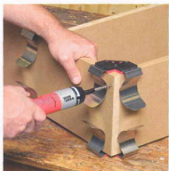
Clever clamps lend a hand. Slip one of these clamps onto a pair of butted boards, and the boards stay put until you're ready to add a clamp or drive a screw.
