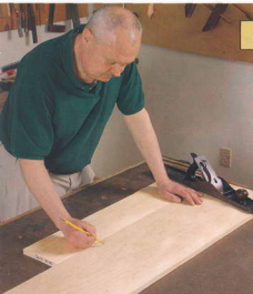
Form the step-back profile. The base is built up by adding a short board to each case side.
