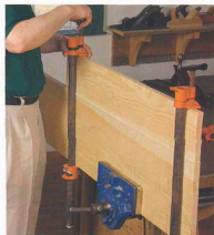
Glue and clamp the two boards. The show side can be handplaned to clean up any tool marks or excess glue.
