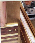
Out of square. The Incra fences weren't square to the table. The problem was fixed by shimming the fence-mounting bracket.
