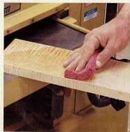
Dampen the board face. Dampening will swell surface fibers slightly, raising short fibers while keeping longer ones flexible.
