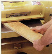
Feed at an angle. Angling the board will keep cutterhead blades from lifting long, undulating wood fibers along the grain.
