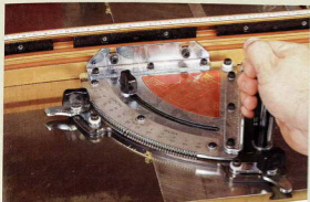
The Incra 2000 can go out of square. If the large black handle loosens with time and use, the fence-support plate will shift slightly left or right.
